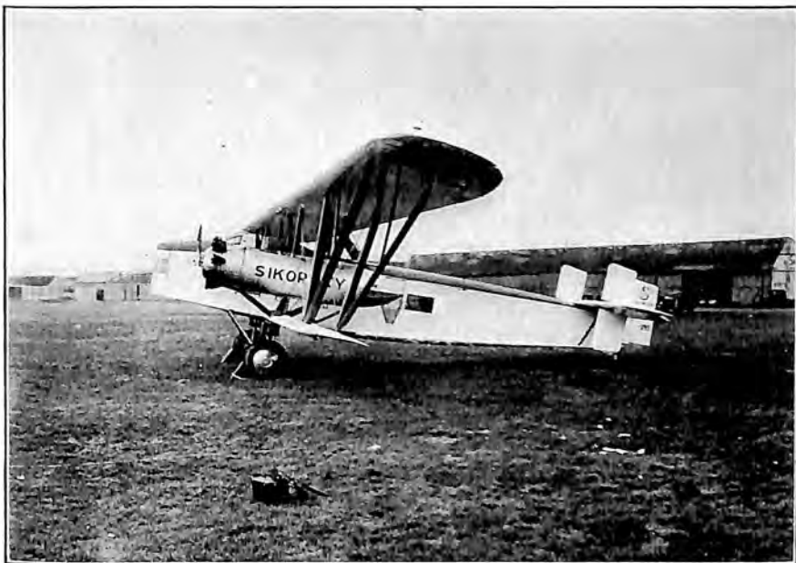
Sikorsky S-37 Commercial. Engines, Gnome Rhone "Jupiter."
