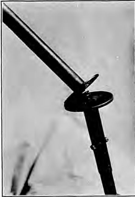
The Alexander Aircraft Company Spring Safety Stick designed to prevent accidents in training due to a student "freezing" to the controls.
