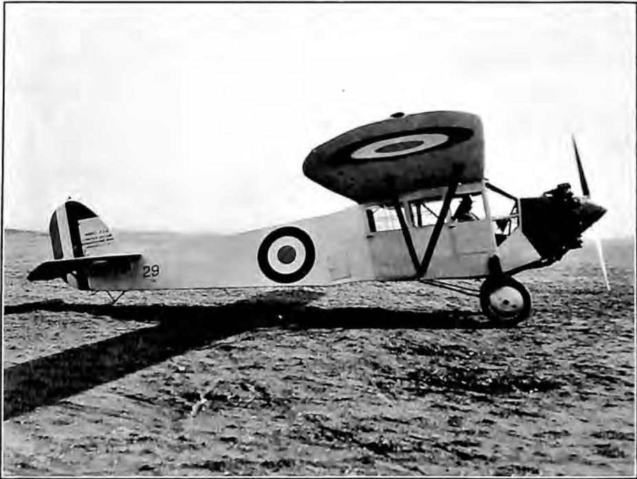
Fairchild All Purpose Airplane. Engine, Wright "Whirlwind."
