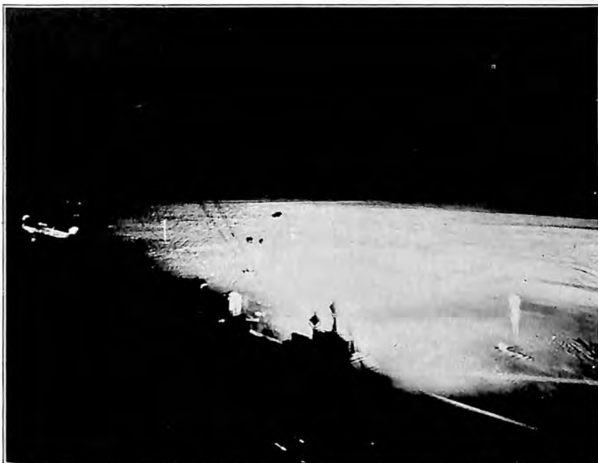
Three Sperry High Intensity Floodlights, fitted with 80° Floodlight Lens, giving full spread of more than 180°, illuminating Airport 3,000 feet square during tests at Wright Field.
