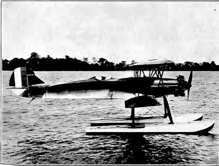
Keystone Seaplane Duster. Engine, "Whirlwind."
