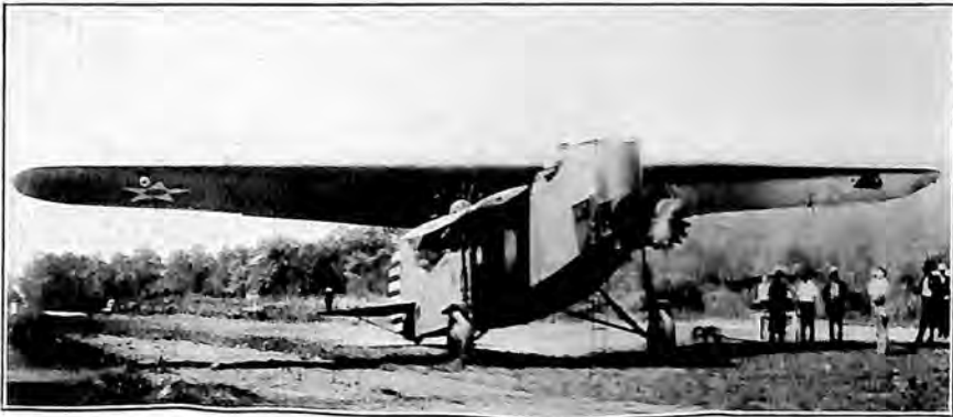
Fokker Twin Army Bomber. Engine, Pratt & Whitney "Hornet."
