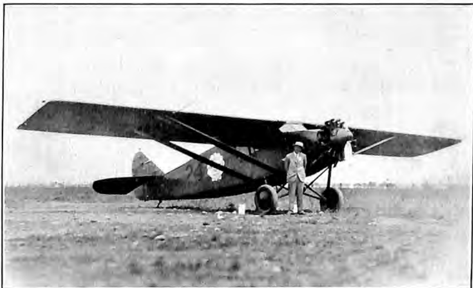
Stinson Monoplane flown by Schlee and Brock, Detroit to Tokio. Engine, Wright "Whirlwind."
