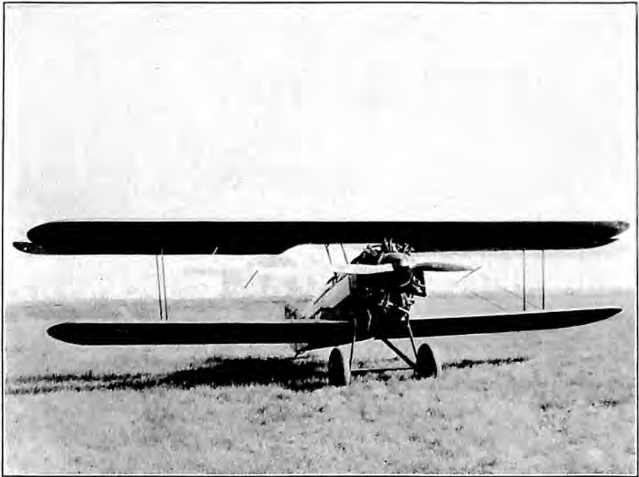
E. M. Laird "Commercial." Engine, "Whirlwind."
